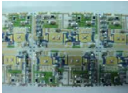
Glue Printing on Populated Substrates
